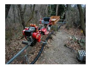
Photo 1.2-4 Monorail used for transporting construction materials.
