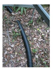
Photo 1.2-7 Unfixed wiring. The forest floor undulates, so it is more practical to use underground corrugated protective tubes for unfixed wiring. (Yamashiro forest hydrology research site)
