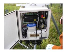
Photo 1.2-13 A measuring box with desiccant (closet dehumidifier) inside.
