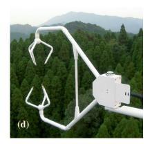
Photo 2.1-1 Configuration of SAT probes: (a) SONIC TR-61C (vertical path, orthogonal probe, Yamashiro forest hydrology research site), (b) ATI "K" Style Probe (vertical path, orthogonal probe, evergreen forest in Kompong Thom Province, Cambodia), (c) SONIC SAT-540 (slanted path, omni-directional probe, evergreen forest in Kompong Thom Province, Cambodia), (d) Campbell CSAT3 (slanted path, boom probe, Kahoku Experimental Watershed).
