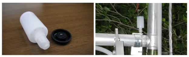
Photo 2.4-2 Air inlet (film canister).
