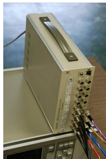
Photo 2.7-1 Low-pass filter for signal cables.
