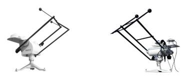
Photo 3.1-3 Measurement of diffuse solar radiation.
