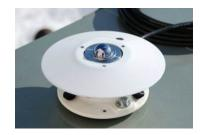
Photo 3.1-4 Infrared radiometers.
