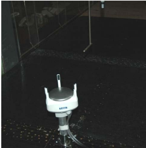
Photo 3.2-2 Inspection of an ultrasonic anemometer in a wind tunnel.
