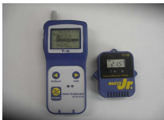
Photo 3.3-2 Ondotori by T&D (thermistor thermometer).
