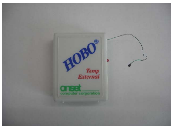
Photo 3.3-1 HOBO by Onset (thermistor thermometer).
