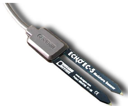
Photo 3.6-1 Permittivity moisture meter EC-5, Decagon. (Photograph: courtesy of Decagon Devices, Inc..)
