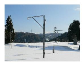
Photo 3.7-2 Snow depth measured by ultrasonic snow gauge. (Tohkamachi Experimental Station)
